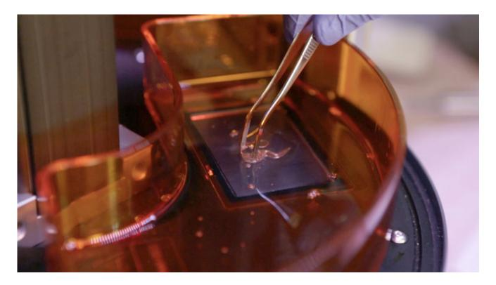
Carefully swipe around the edges of the resin tray window and remove any build up.
