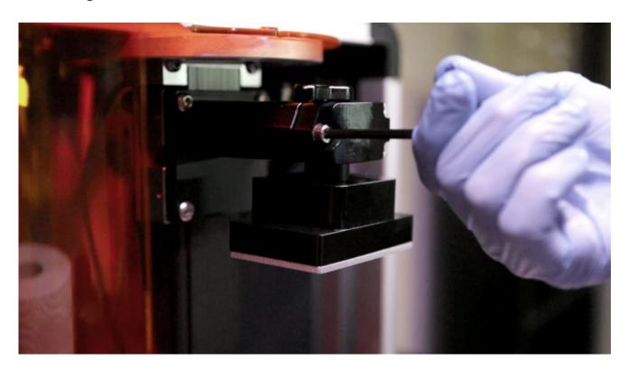
We'll need to relevel the build head before starting a new job - mainly because it misaligns after removal. So we can loosen a the build plate and move it up, and then we'll tighten up the screw.
