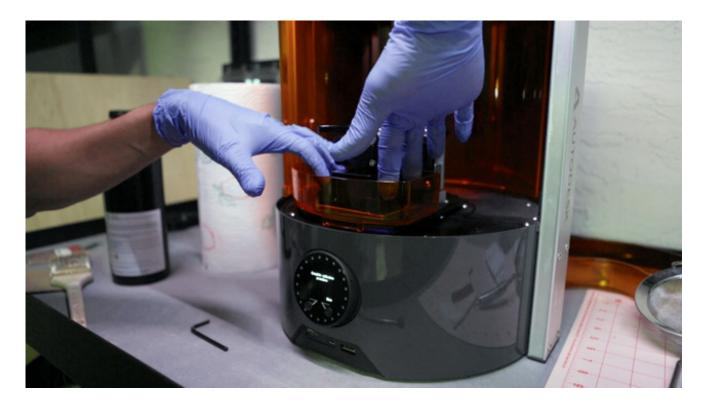
From here we can loosen the build head - let it drop down and push on all four corners to lay it flat. Once its all straight and level, we can tighten it back up and complete the process.
