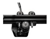
5. Lock the X-axis limit assembly on the XE axis with two M4x8 hexagon socket head cap screws.
