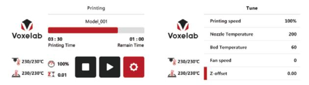
When the offset value is positive, the nozzle and the build plate gets farther; When the offset value is negative, the nozzle and the build plate get closer.
