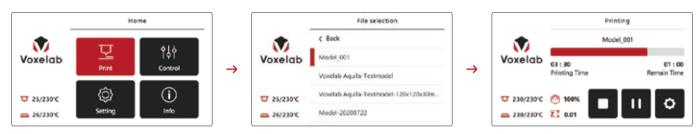
Note: When you notice the improper distance between the nozzle and the build plate during printing the first layer, please click the setting button to perform the z-axis offset.
