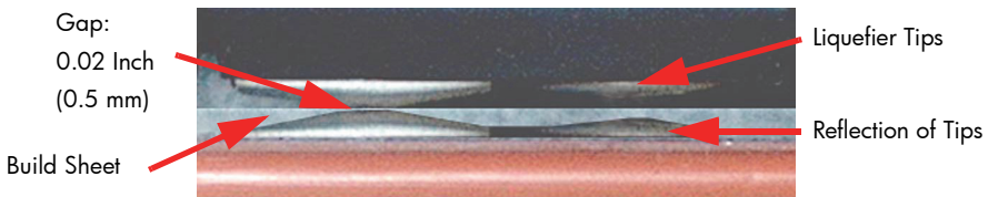
Figure 6-3: Manual Z Zero Calibration
